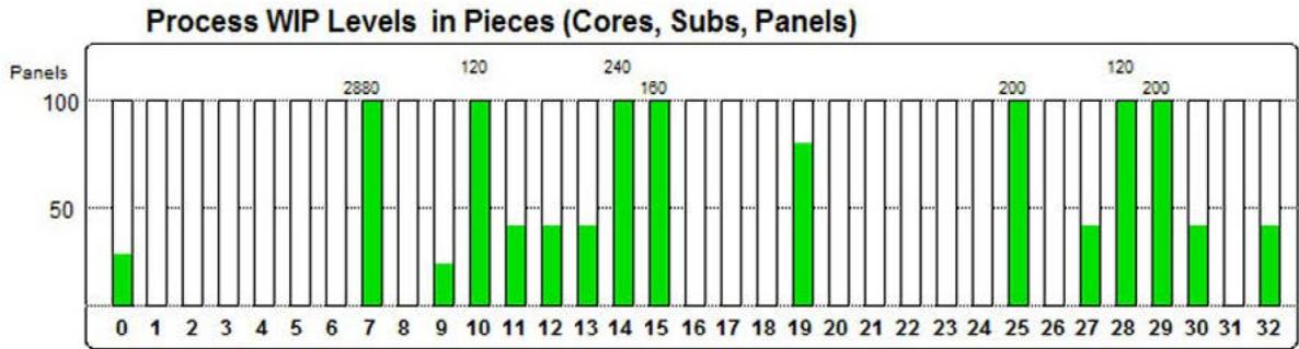
Figure 1: Capacity result with infrequent large lots. Each department is labeled and numbered. The numbers correspond to the number on the Process WIP levels graph. The green squares show which departments were processing panels at the end of the simulation and the green bars show the WIP levels, which can help to identify bottlenecks.
