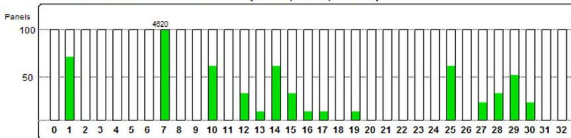
Figure 2: Capacity result with frequent small lots. Each department is labeled and numbered. The numbers correspond to the number on the Process WIP levels graph. The green squares show which departments were processing panels at the end of the simulation and the green bars show the WIP levels, which can help to identify bottlenecks.
